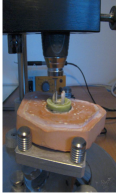
Fig 2. Preparing the cavities inside the teeth with a parallelogram. In these cavities the different filling materials were placed
